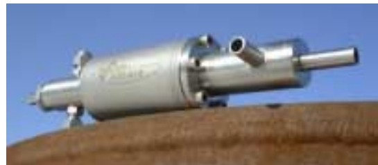
Fig. 7 Ejector dilutor (left side: drawing of the Palas-system, right side: picture of the system, manufactured by Dekati)
