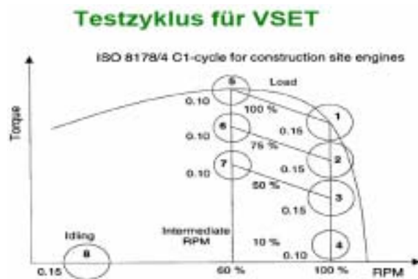
Fig.1. Test Cycle for Secondary Emissions Test. Only test modes 1, 3, 5 and 7 and engine mode for high filter space velocity is needed for PFS filtration evaluation
